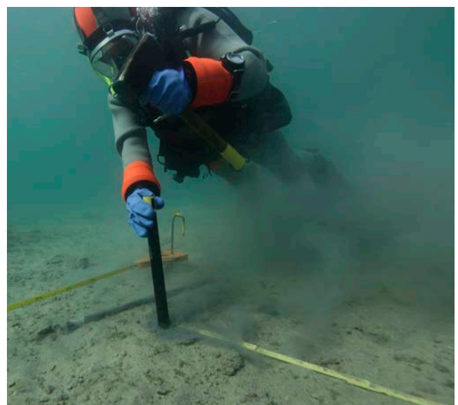
Fig. 3 Diver placing an erosion marker at Thun, Schadau, Lake Thun. It is a cost-effective and efficient method to measure the erosion rate of the lake bed over the long term © Archaeological Service of the Canton of Bern, Carlos Pinto, 2016.
