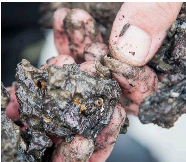
Fig. 1 In saline water the attack of Teredo navalis (shipworm) is an enormous threat to shipwrecks and other wooden structures. Here we can see the devastating effect the shipworm has on historical shipwrecks. The wood has crumbled and almost disappeared. © Paul Voorthuis, High Zone Photography.
