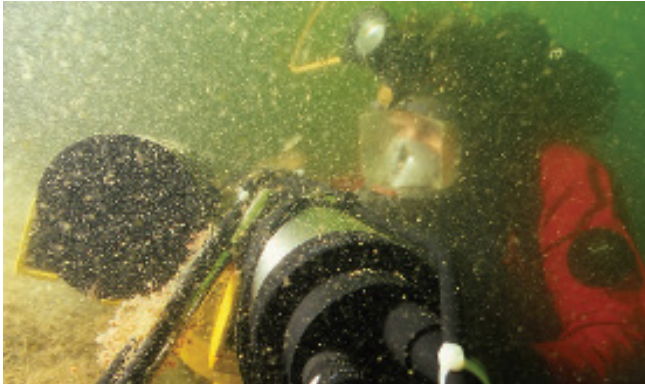
Fig. 5 A diver with a data-logger. This equipment measures parameters such as conductivity (salinity), dissolved oxygen, and current strength. Diver or remote sensing can also monitor physical changes to sites which can be applied to natural environmental and cultural purposes. It can help us to see the changes in the site and detect or predict threats. Photo: BZN 10 wreck - the Netherlands. © RCE.
