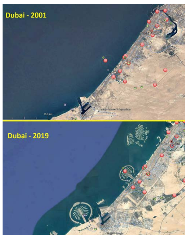
Fig. 2 Dubai UAE: the difference in the country's coast line between 2001 and 2019 as a result of the infilling. Map data 2001: Image Landsat / Copernicus © Google 2019: Image Landsat / Copernicus © Google Data SIO, NOAA, U.S. Navy, NGA, GEBCO.
